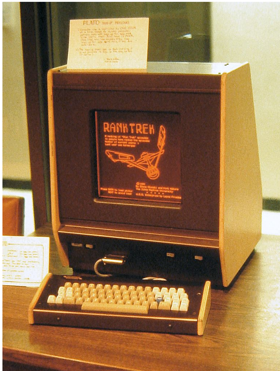
Figure 2.1: The microprocessor-based PLATO V terminals for the PLATO IV system featured plasma displays, infrared touch panels, and local processing capabilities. (Photography contributed to Wikipedia by user Mtnman79 and licensed under the Creative Commons Attribution 3.0 License)
